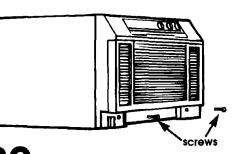
**20** Attach front by first removing the two, #8 x 9.5 mm (3/8") screws from base; then insert front tabs into top of cabinet and swing front in place. Attach bottom of front by reinserting the two screws.
